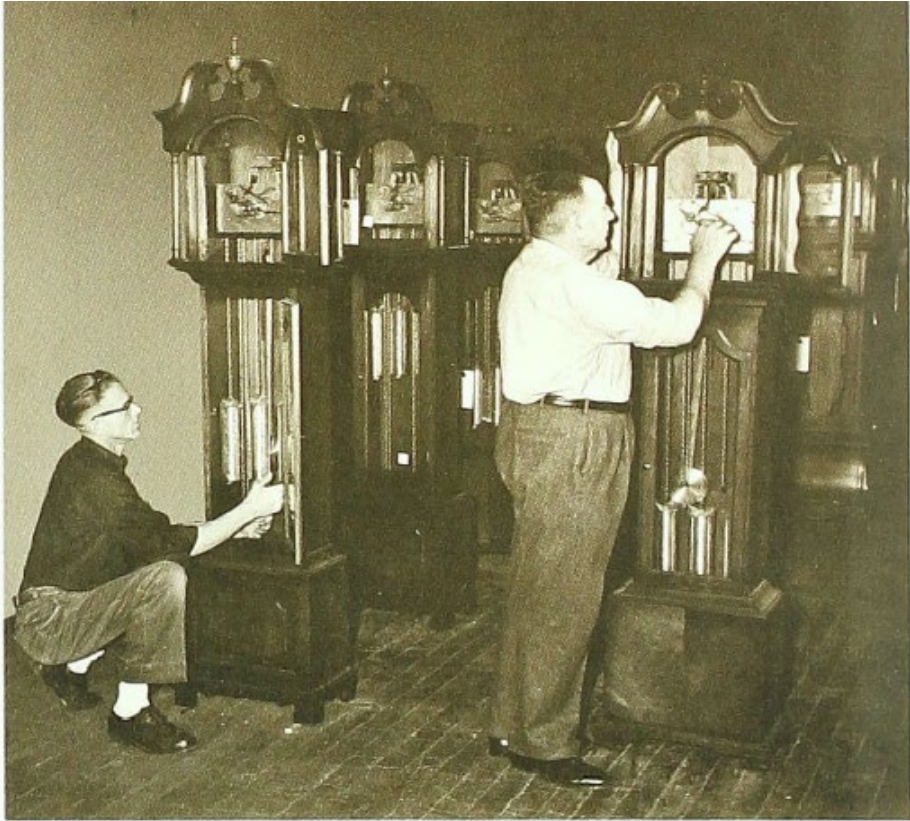
Final inspection, adjustment and assembly of clock movements into finished Colonial cases.
